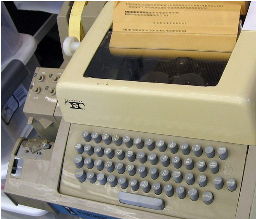
A Teletype Model 33 ASR with paper-tape punch and reader.
