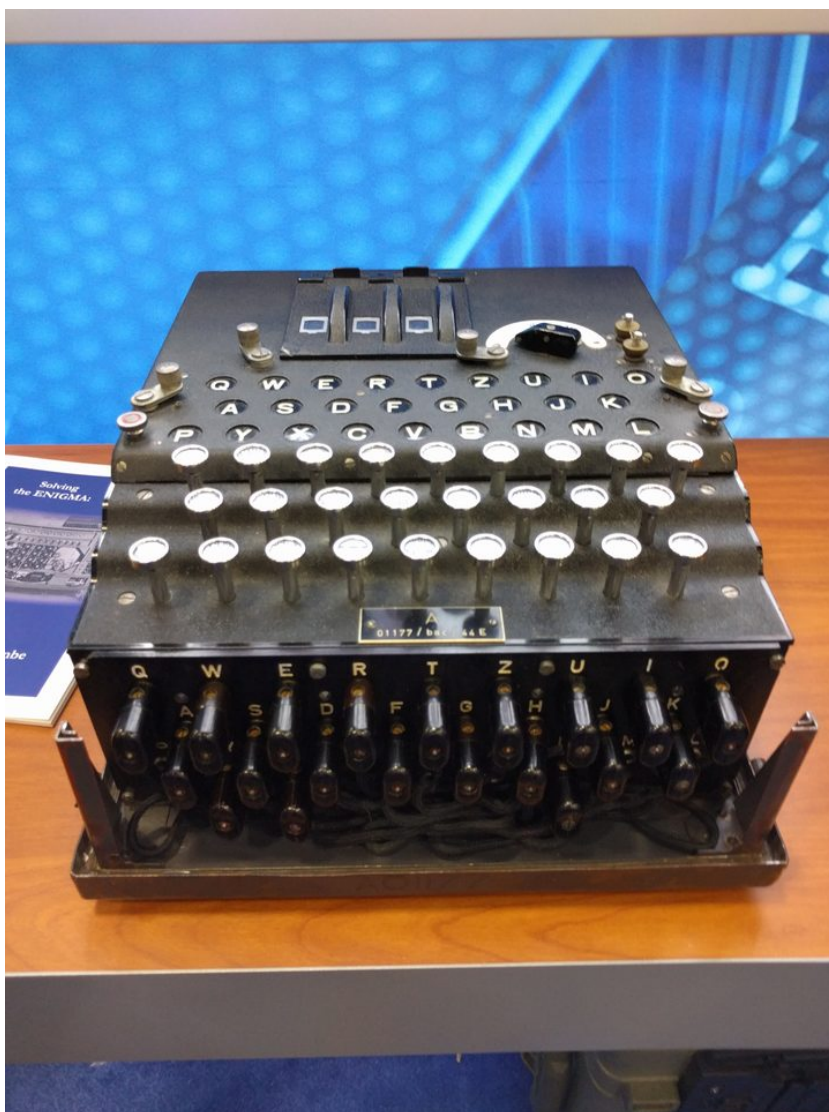
An Enigma machine with its keyboard, lampboard, plugboard and three rotor windows visible.
